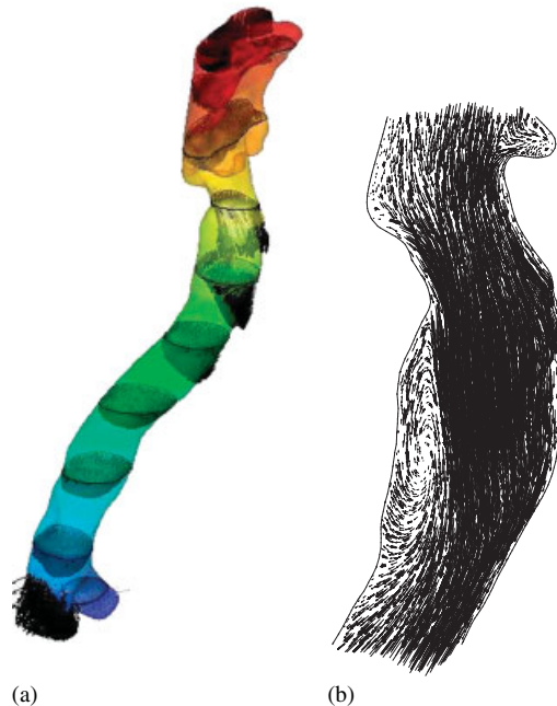
Figure 12. Velocity vector plots at an inhaling flow rate of 33.761\text{l}/\text{m} : (a) vectors and (b) recirculation below the vocal cords.
